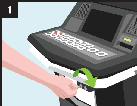
INSERT AND TURN RESET KEY (TO CANCEL CREDIT)
